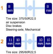
Tire size: 295/60R22, air suspension Disc brakes
